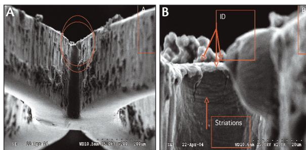
Figure 2. Scanning electron micrograph of a commercially available stent showing cracks, striations, and retained slag.
