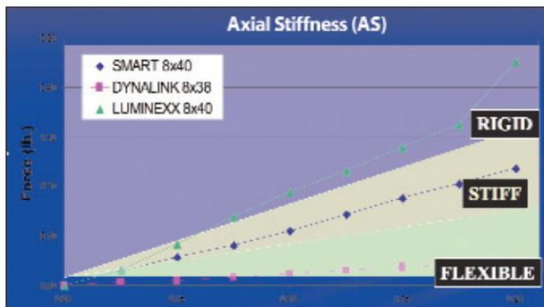
Figure 3. Three commercially available stents with different axial rigidities.
