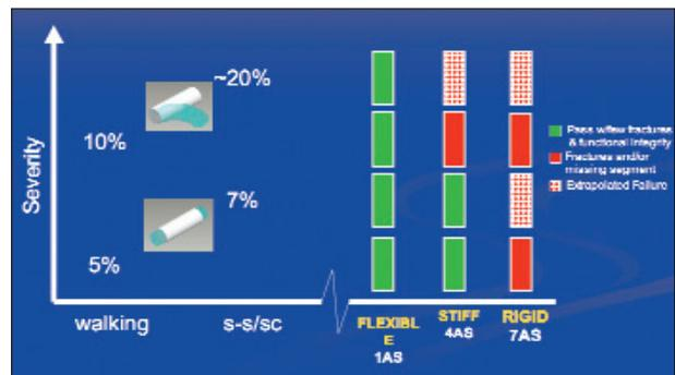
Figure 4. Fatigue resistance is significantly better with axially flexible stents.
